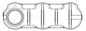
OVERFLOW CAN BE FITTED AT EITHER END 3 X 25MM MOULDED BRASS OUTLETS
