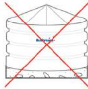
Rocky and uneven ground with little or no base preparation.
